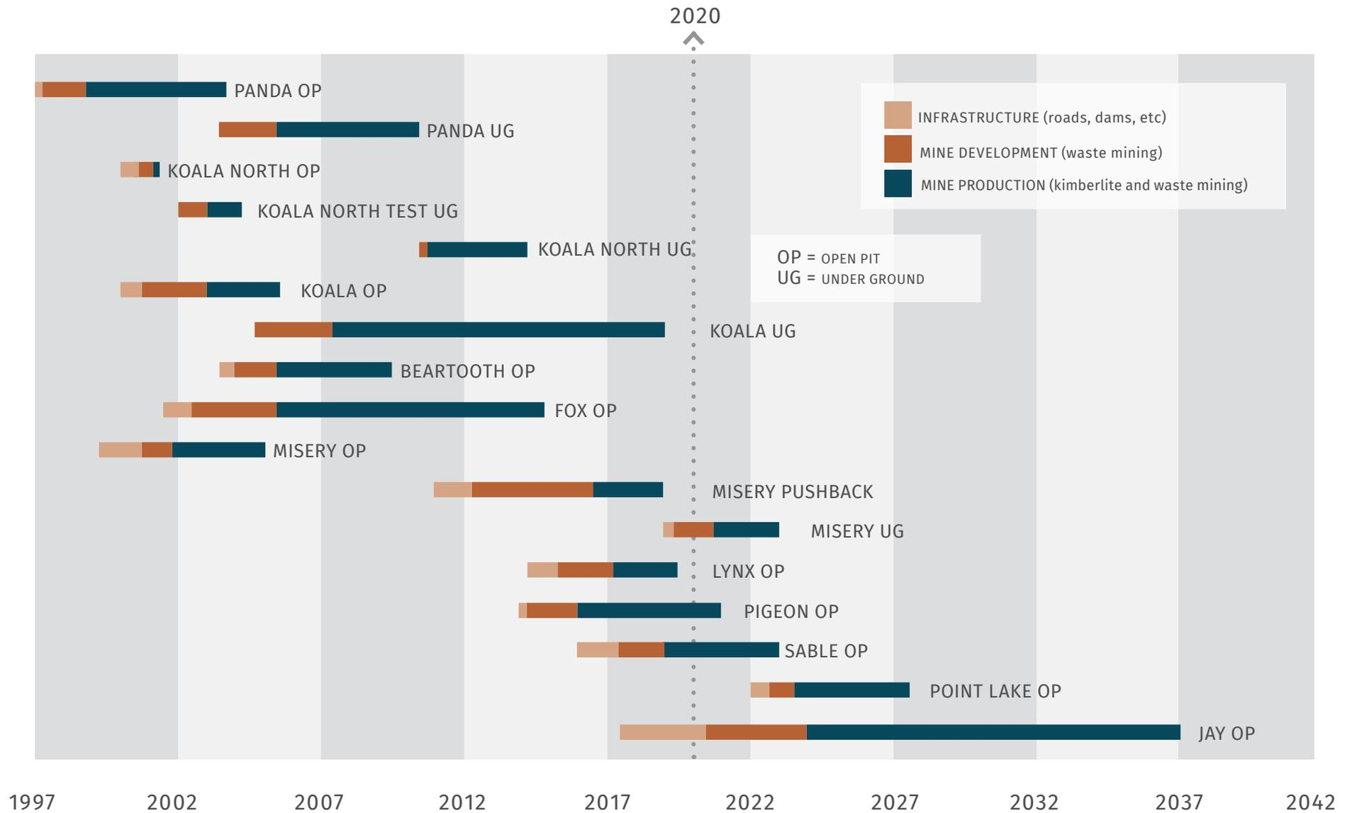
Figure 1: The Ekati Diamond Mine: Life of Mine Plan
