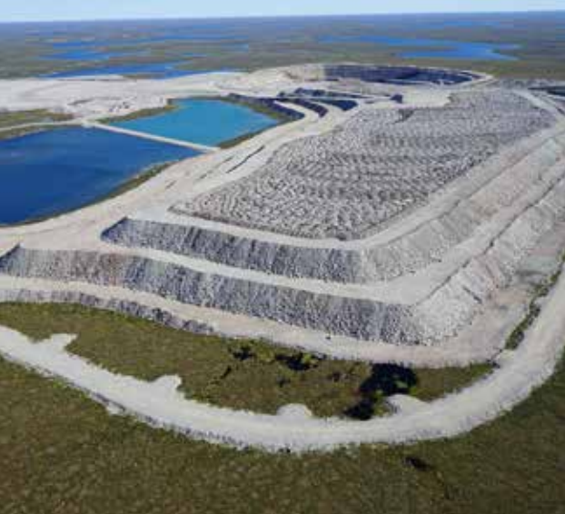
Sable operations with waste rock pile, two-rock sedimentation pond and pit in distance - photo courtesy of Ekati Diamond Mine.
