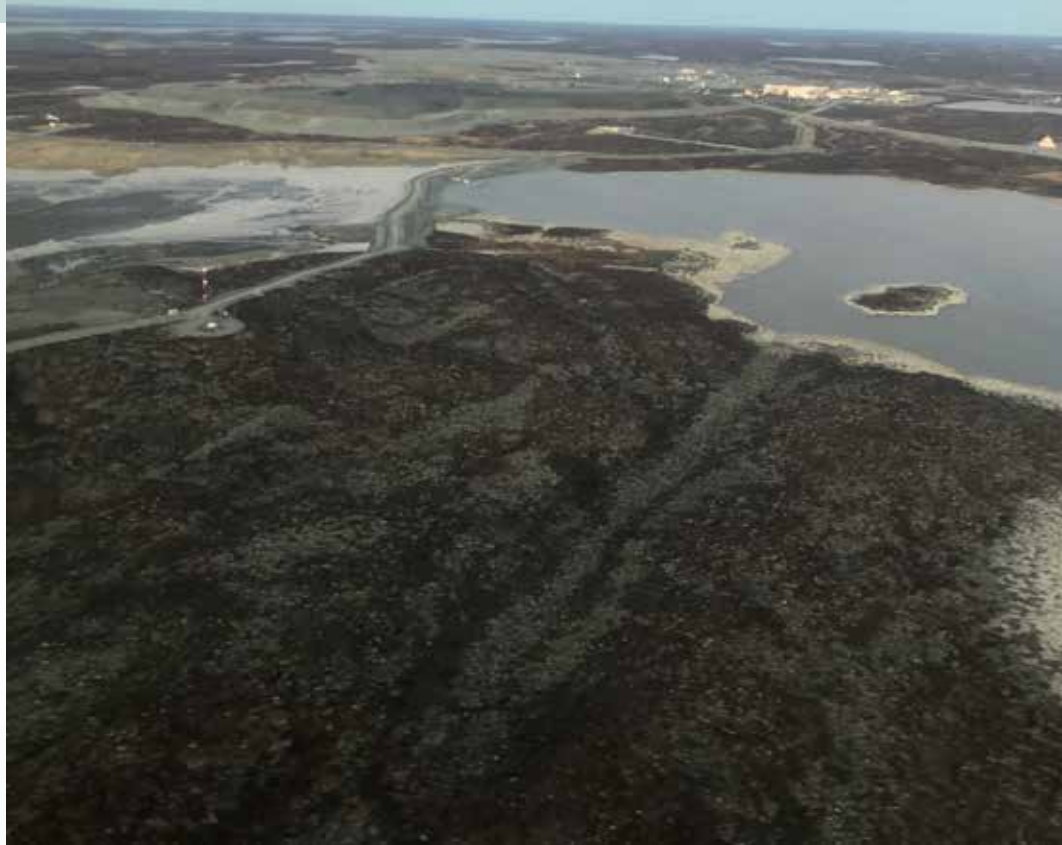
Dyke C separating Cell C with Processed Kimberlite on left from Cell D with open water on right
