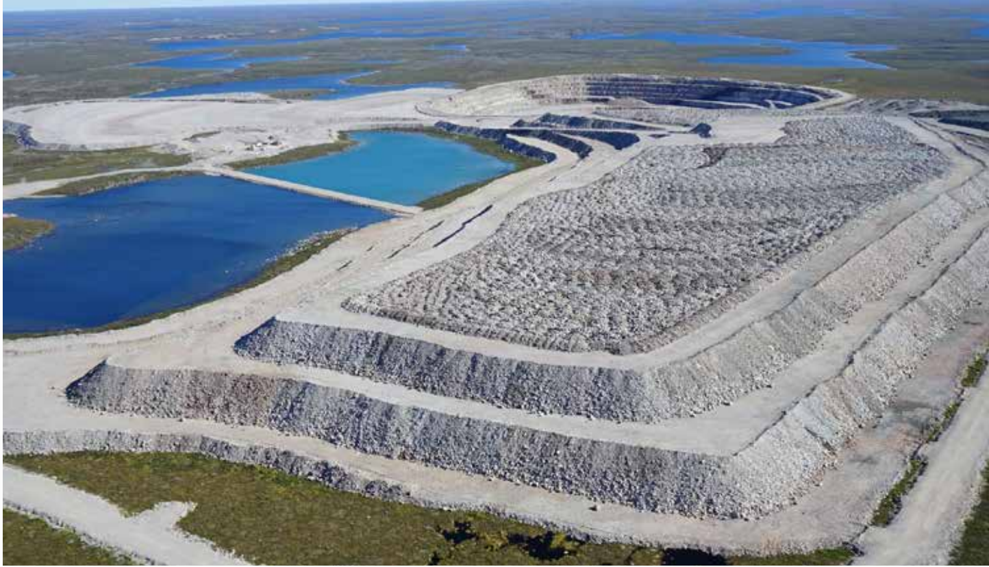
Sable Waste Rock Pile, Open Pit and Two-Rock Sedimentation Pond photo courtesy of Ekati Diamond Mine.
