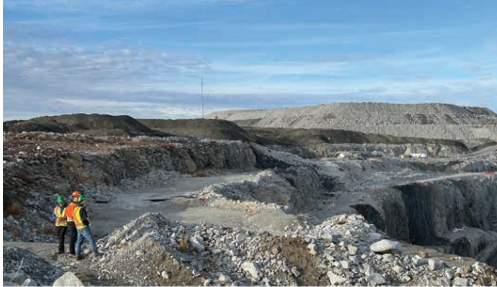
Misery Pit with low grade kimberlite (dark rock) and WRSA in the background
