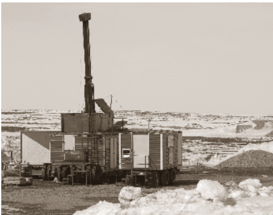
Diamond drill rig at Pigeon Pipe.
