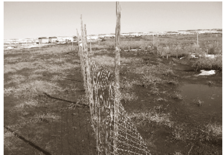
Enclosed revegetation test plot on cell B.
