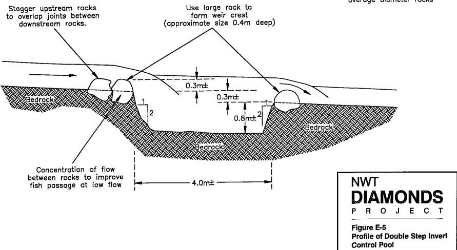
recommended as a stream channel improvement measure (Kerr et al 1980). The general purpose of this structure is to provide resting places for fish within sections of swifter moving water. DSIC pool dimensions and substrate
